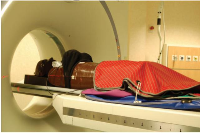
**Figure 1.** Experimental set-up showing the RANDO phantom, the positioning of the lead aprons and clearly demonstrating the folds and gaps in the aprons.
