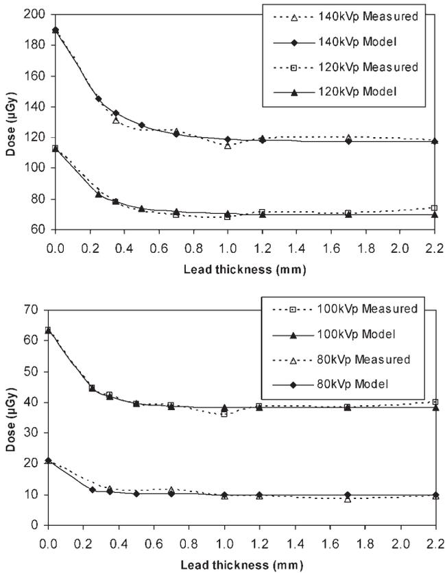
**Figure 3.** (a) Experimental data and modelled data for tube potential settings of 140 kVp and 120 kVp. (b) Experimental data and modelled data for tube potential settings of 100 kVp and 80 kVp. Errors on all values in Figure 3 are 1%.
