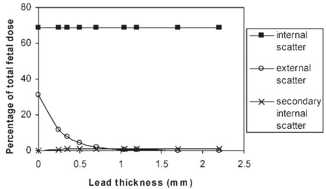
**Figure 4.** The relative contributions of the three sources of scattered radiation to the total fetal dose as calculated using the proposed model at 140 kV<sub>p</sub>. (The indicated dose levels are illustrative, as the exact values will vary from scanner to scanner.)
